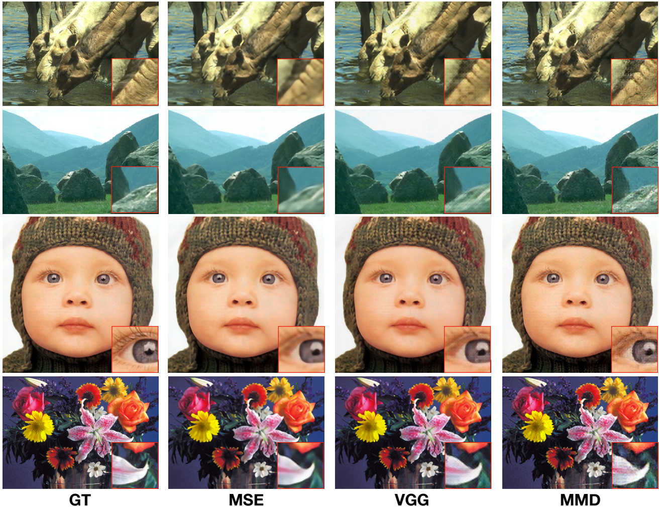
Figure 4. Qualitative comparison of image super-resolution results for different loss functions. Our new loss clearly produces sharper results than both MSE and VGG based perceptual loss, while also producing less artifacts than the VGG loss.
