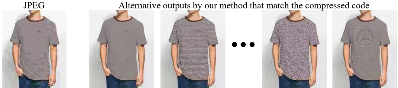
Figure 1. Ambiguity in JPEG decomposition. A compressed JPEG file can correspond to numerous different plausibly looking images. These can vary in color, texture, and other structures that encode important semantic information. Since multiple images map to the same JPEG code, any decoder that outputs only a single reconstruction, fails to convey to the viewer the ambiguity regarding the encoded image.
