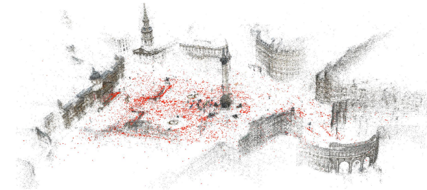
Figure 1. Reconstructions generated from the Trafalgar dataset [45], where 7085 out of 15685 images have been registered, and the rotation averaging step only took 4.2 s.
