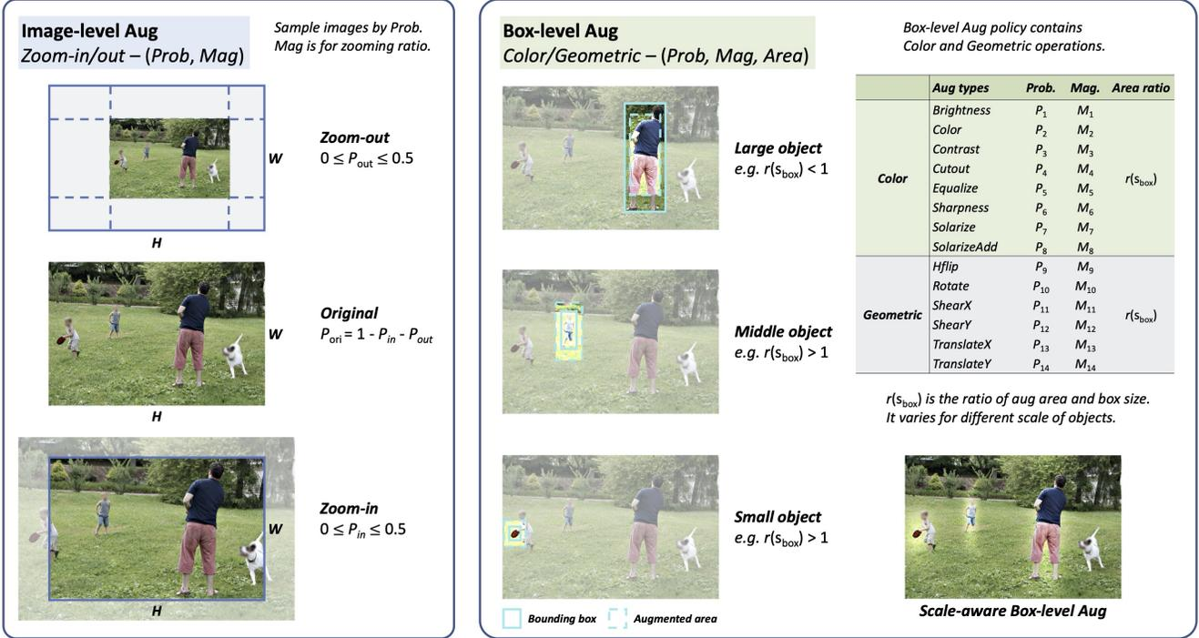
Figure 2: Scale-aware search space. It contains image-level and box-level augmentation. Image-level augmentation includes zoom-in and zoom-out functions with probabilities and magnitudes for search. In box-level, we introduce scale-aware area ratios, which make operations adaptive to objects in different scales. Augmented images are further generalized with the Gaussian map.
