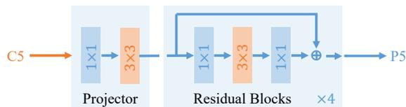
Figure 5. An illustration of the structure of *Dilated Encoder*. In the figure,  $1 \times 1$  and  $3 \times 3$  denotes  $1 \times 1$  and  $3 \times 3$  convolution layers and  $\times 4$  means four successive residual blocks. All convolution layers in Residual Blocks are followed by a batchnorm layer [12] and a ReLU layer [24], while in Projector, we only use convolution layers and batchnorm layers [12].
