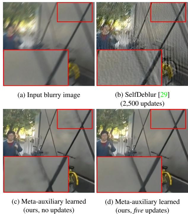
Figure 1: Sample deblurring results. Given a blurry input image (a), SelfDeblur [29] requires thousands of iterations to learn the internal information of the input image (b). Our approach uses meta-auxiliary learning to learn to adapt to the unique properties of the given image. Before adaptation, the output has some artifacts due to the distribution shift between the training dataset and the test image (c). After five updates, our model quickly adapts to the internal information of the test image and removes the artifacts (d).
