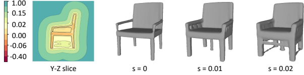
Figure 3. The learned template implicit field (Y-Z slice) for chair category and different iso-surfaces extracted from it. Note that the template implicit field is not a valid shape SDF and it characterizes different shape structures within a category.
