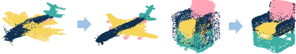
Figure 8. Labeled points on the original shapes are deformed into the template 3D space where the semantic parts are well aligned
