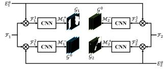
Figure 4. **Group collaborating module.** The original feature maps and consensuses of both groups are fed to the GCM. The predicted output conditioned on the consistent feature and consensus (from the same group) is supervised with the available ground-truth labels. Otherwise, it is supervised by the all-zero maps.
