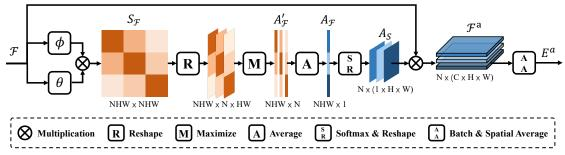
Figure 3. **Group Affinity Module.** We first exploit the affinity attention to generate the attention maps for the input features by collaborating all images in group. Subsequently, the maps are multiplied with the input features to generate the consensus for the group. Then the obtained consensus is used to coordinate the original feature maps and is also fed to the GCM for inter-group collaborative learning.
