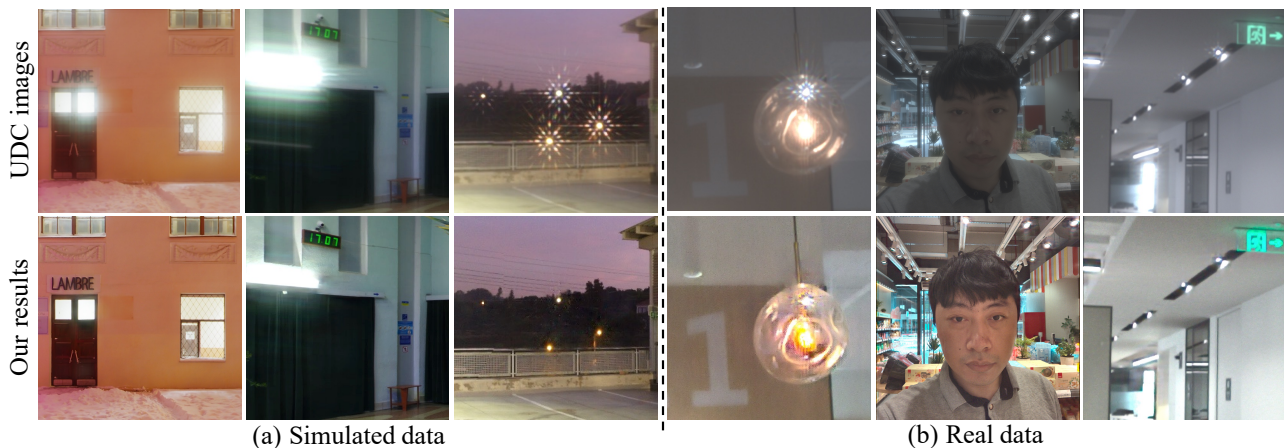
Figure 1. Removing Diffraction Artifacts from Under-Display Camera (UDC) images. The major degradations caused by light diffraction, e.g. , flare, blur, and haze, could significantly affect the visual quality of UDC images. Our method effectively restores fine details and suppresses the diffraction effects of UDC images.
