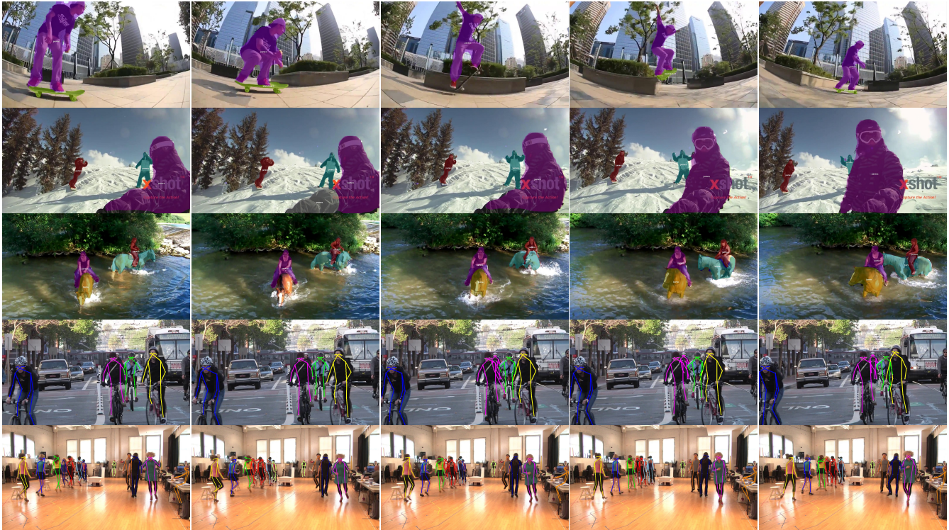
Figure 4. Visualization results of our proposed semi-supervised tracking approach on video instance segmentation and pose tracking. Each row has five sampled frames from a video sequence. Categories, bounding boxes and instance masks are shown for each object. Note that objects with the same predicated identity across frames are marked with the same color. Zoom in to see details.
