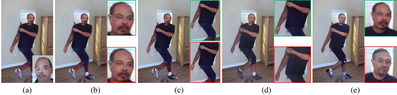
Figure 5. B2F/FR ablation study. (a) Our result and the target face. In the following, we show the resulting frame of a variant of our method. In red a zoom in of a certain part, and in green the same crop from our full method. (b) No FR ( blurrier face, features are less distinctive ), (c) no blending mask ( crude edges surrounding the entire rendered character ), (d) hand/finger labels not added ( arm distortions due to finger uncertainty, fingers less distinct ), (e) no face loss, lower resolution (256x160) ( appearance not preserved, edge pixelization )
