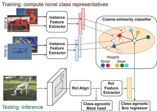
Figure 1. **Incremental few-shot instance segmentation.** For all  $K$  instances of each novel class, we produce vector embeddings using an Instance Feature Extractor. The average of these embeddings is stored as a per-class weight vector inside a cosine-similarity classifier. At test time (green), we compare the cosine distance embeddings of object proposal to the per-class weights.
