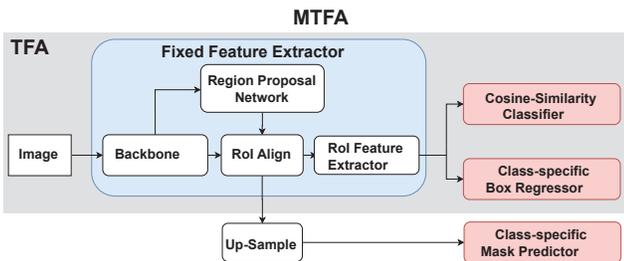
Figure 2. **Architecture of TFA and MTFA.** MTFA extends TFA with a mask prediction branch. In the first training stage, the whole network is trained on the base classes. In the second stage, the feature extractor is frozen (blue) while the classifier and box and mask heads (in red) are fine-tuned on base and novel classes.
