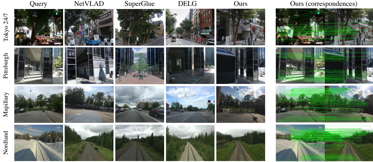
Figure 5. Qualitative Results. In these examples, the proposed Patch-NetVLAD successfully retrieves the matching reference image, while NetVLAD, SuperGlue and DELG produce incorrect place matches (except Tokyo where DELG also finds the correct match). The Tokyo 24/7 match example is particularly challenging, with a combination of day vs night-time, severe viewpoint shift and occlusions.
