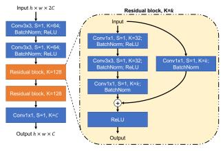
Figure 4: The two residual blocks are trained to refine the segmentation at each scale. This module outputs the same size  $h \times w$  as the input.
