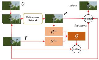
Figure 3: The overview of the refinement module. The cumulative segmentation Y is partly replaced with the scale-specific segmentation map O based on the score  $\mathcal{Q}$ .
