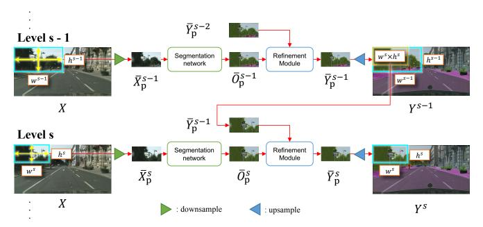
Figure 2: **Overview of our proposed MagNet**. The segmentation network produces the scale-specific prediction while the refinement module selectively refines the coarse prediction from previous stages based on that local prediction.
