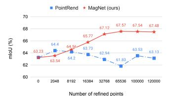
Figure 7: Correlation between the number of selective points of each scale and mean IoU on the Cityscapes dataset. When the quantity of points increases, the performance of MagNet continuously grows while the mIoU of PointRend decreases.
