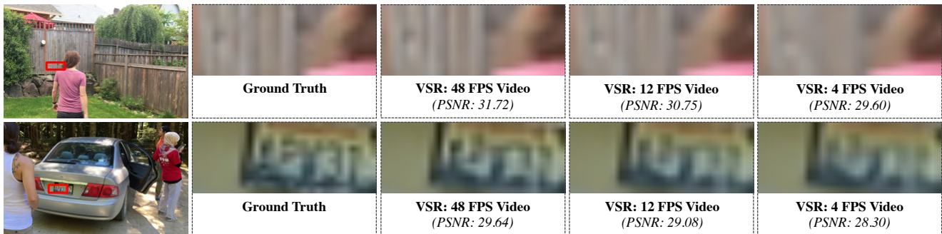
Figure 1. Influence of temporal frequency on the performance of VSR. A higher frame rate, and hence a smaller displacement between consecutive frames, yields enhanced VSR results obtained by a state-of-the-art approach [53], as evidenced by the rising PSNRs.
