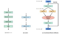
Figure 2. (a) Lite  $3 \times 3$  is the most basic building block. (b) Lite k consists of  $\lfloor \frac{k}{2} \rfloor$  Lite  $3 \times 3$ . (c) CBlock combines two kinds of kernel  $(k_1, k_2)$ , and C  $\times$  H  $\times$  W denotes the current shape of the tensor.
