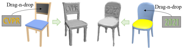
Figure 8. When a logo image, e.g., of “CVPR”, is “drag-n-dropped” onto a chair image, we obtain a reconstructed 3D chair model (shown in a view that is different from that of the input image) with surface features resembling the input logo.
