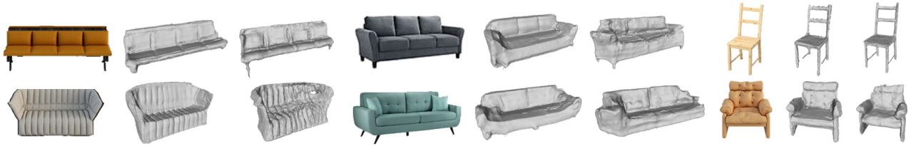
Figure 7. Reconstruction results from single-view images “in the wild” using D^2IM-Net (left) and D^2IM-Net_{GL} (right).
