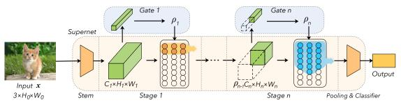
Figure 3. Architecture of DS-Net. The width of each supernet stage is adjusted adaptively by the slimming ratio  $\rho$  predicted by the gate.
