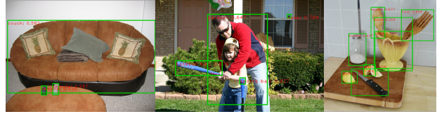
Figure 2. Some samples to show the co-occurrence of both base and novel classes in the same image according to the commonly used dataset setting for MS-COCO, “couch”, “person” and “bottle” are novel classes while the others are base classes. Due to incomplete annotations, those novel-class objects can be unlabelled in base set.
