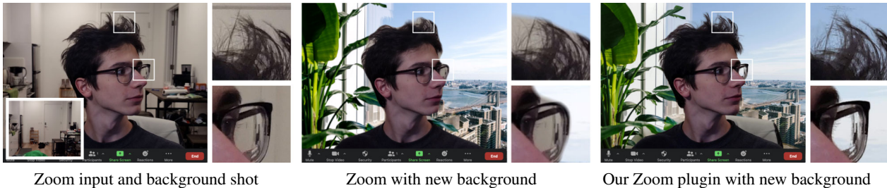
Figure 1: Current video conferencing tools like Zoom can take an input feed (left) and replace the background, often introducing artifacts, as shown in the center result with close-ups of hair and glasses that still have the residual of the original background. Leveraging a frame of video without the subject (far left inset), our method produces real-time, high-resolution background matting without those common artifacts. The image on the right is our result with the corresponding close-ups, screenshot from our Zoom plugin implementation.
