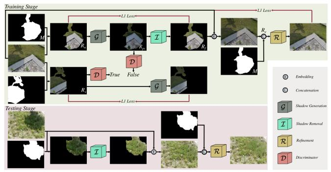
Figure 2. The network architecture of our proposed G2R-ShadowNet. It takes in a shadow image and its corresponding shadow mask to produce the shadow-free result in the shadow regions. The training stage involves all the three sub-nets of shadow generation, shadow removal and refinement, while the testing stage does not perform shadow generation.
