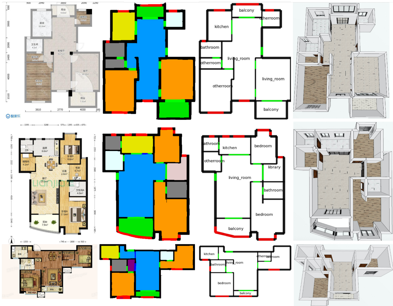
Figure 3. Floor plan recognition and reconstruction results. From left to right, an input floor plan image, semantic segmentation result with post-processing, reconstructed vector-graphics representation with room type annotation, the corresponding 3D reconstruction model. The original images come from Kujiale [4] (top), Lianjia [5] (middle) and Fangtianxia [2] (bottom).
