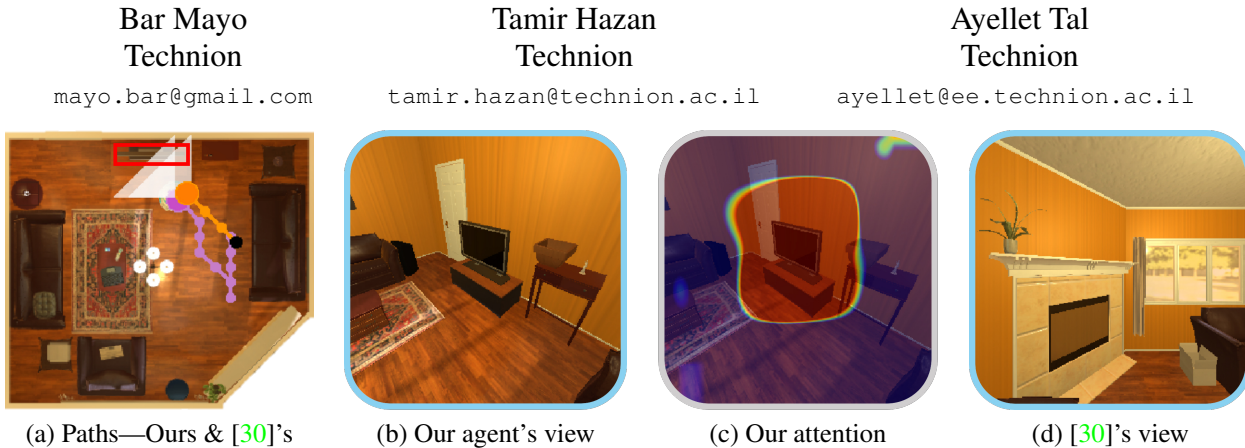
Figure 1. Visual navigation. (a) The agent aims at finding a TV (red rectangle) in a living room (top view), starting from a given location (black circle). Our agent’s path is marked in orange and [30]’s path is in magenta. At each step, the agent is given a specific view, depending on its position. In this example, our agent starts by turning around in its starting location to gather information—a strategy it has learned. (b) shows our agent’s view before the first move forward, whereas (d) shows [30]’s view before its first move forward. (c) shows our attention model, which combines semantic and spatial information of (b)’s view; it directs our agent to move forward, towards the TV. Differently, the view in (d) is part of [30]’s lengthy exploration (magenta path in (a)) after the sought-after TV.
