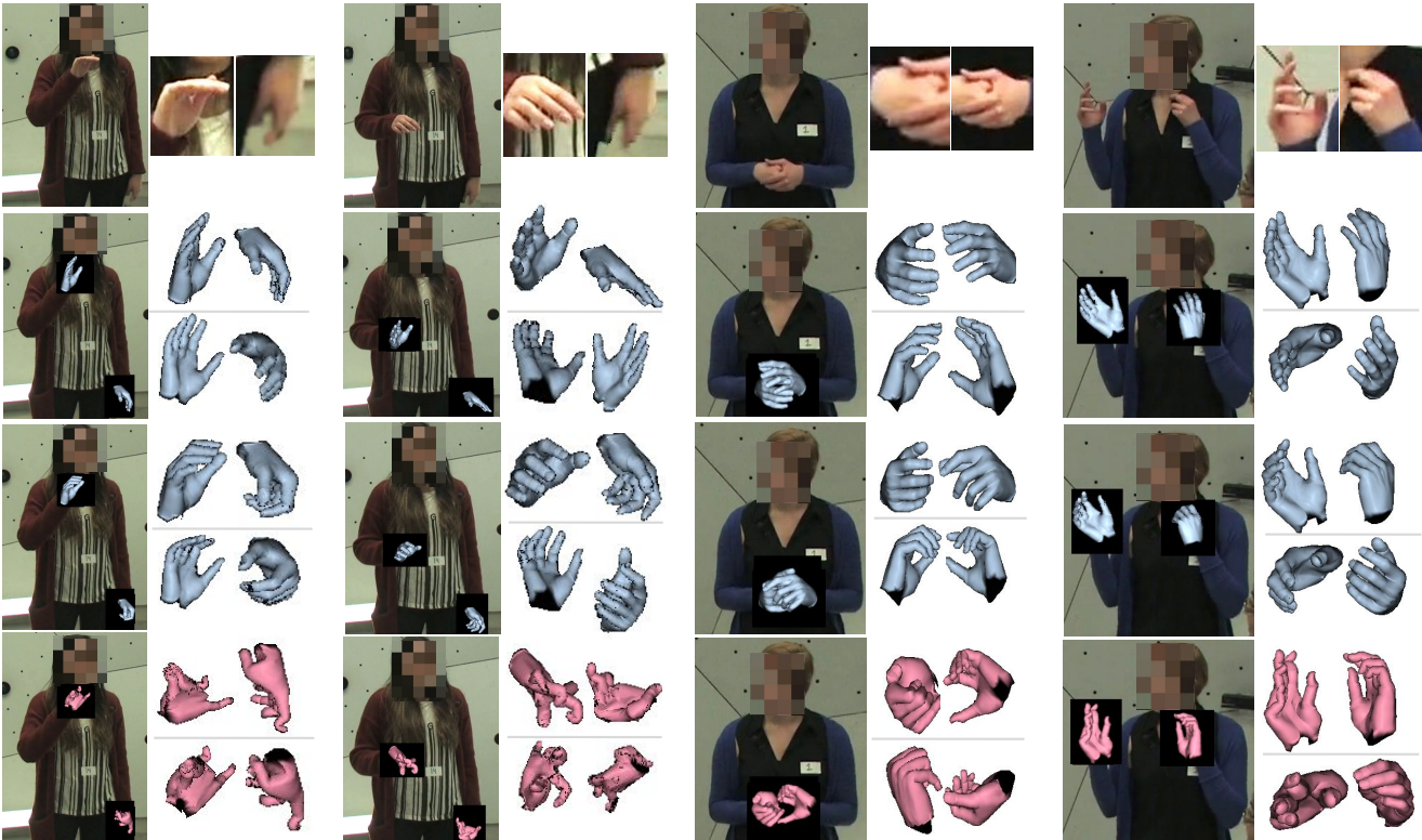
Figure 6. Adding the image embedding improves the accuracy for examples where using the body prior alone fails due to low/no distinguishable body motion. We show two views for each prediction below their respective hands. Row 1: View of speaker and magnified hands. Row 2: Our results from using body prior alone. Row 3: Adding an image feature with the prior addresses this issue, snapping to the true hands. Row 4: MTC [51] image-based results. Shown are “unclear” frames as referred to in Tab 1. See video for all frames.
