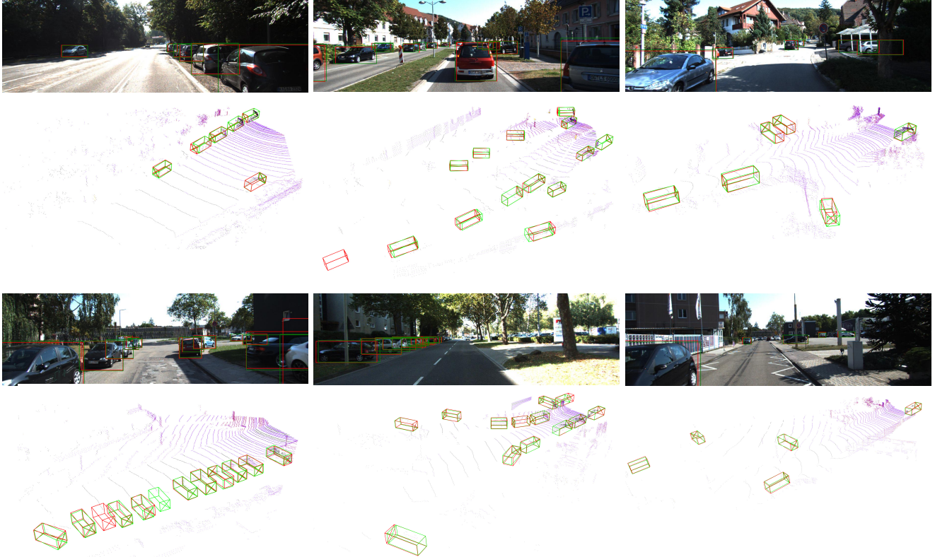
Figure 4: Qualitative results on the validation split of KITTI [10]. Our predictions and ground-truth bounding boxes are shown in green and red, respectively. Our method localizes small and/or occluded objects well, except the heavily occluded ones, e.g. , in the left-bottom of the top-middle image. We also show 2D bounding boxes projected from 3D detection results. Best viewed in color.
