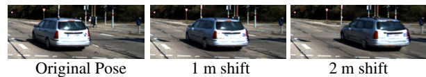
Figure 6: A learned vehicle leaf node is translated by 2 meters perpendicular to the movement observed during training. The model changes the shadows and specular highlights on the vehicle consistent with learned global scene illumination.
