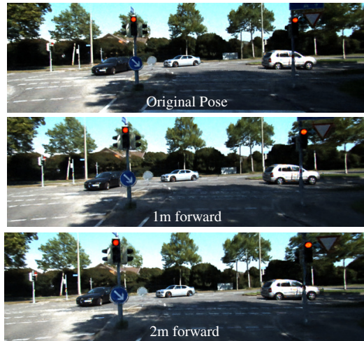
Figure 8: Unseen view synthesis results. Here we move the ego camera by approximately 2 m into the scene with all other nodes of the scene graph fixed. The method accurately handles occlusions from traffic lights and signs, highlighting the capabilities of the proposed scene graph for novel view synthesis.
