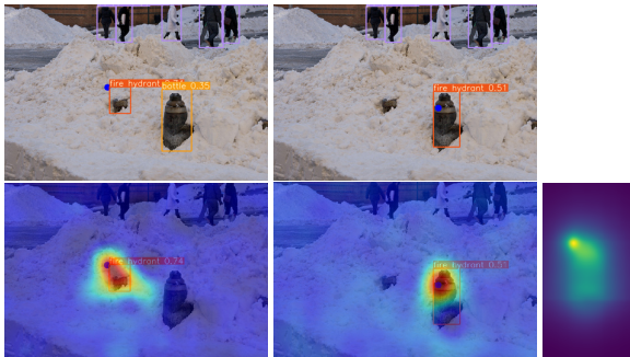
Figure 7: We train YOLOv3 on a biased dataset, in which a blue dot is placed precisely at the top left corner of every bounding box containing a fire hydrant. At test time, we can move the blue dot arbitrarily. We notice that the presence of the dot can trigger false positives (background being mistaken for a fire hydrant in top-left) and produce misclassifications (a fire hydrant detected as a bottle in top-right). Corresponding saliency maps produced by D-RISE correctly point to the blue dot as a reason for these errors, and the average saliency map (bottom right) shows a significant artifact on the top-left corner. This type of analysis can provide model designers or data scientists with insights about pathological biases in the dataset.
