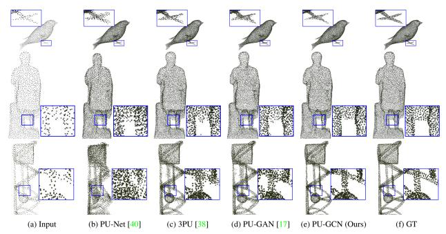
Figure 5: **Qualitative upsampling results.** We show the  $\times 4$  upsampled results of input point clouds (2048 points) when processed by different upsampling methods (PU-Net, 3PU, PU-GAN and our PU-GCN). PU-GCN produces the best results overall, while generating less outliers and preserving fine-grained local details (refer to close-ups).
