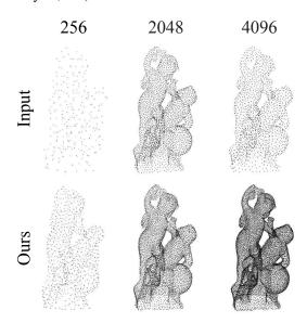
Figure 8: **Effect of input size.** The top row shows the input point clouds of different sizes, and the bottom row shows the ×4 upsampled outputs of our PU-GCN. PU-GCN always produces high quality results regardless of input size.
