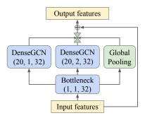
Figure 3: **Multi-scale feature extractor: Inception DenseGCN.** We use the parameters (k, d, c) to define a DenseGCN block. k is the number of neighbors (kernel size), d is the dilation rate, and c is the number of output channels. Green  $\bowtie$  denotes feature-wise concatenation. Note that the d is different in the different DenseGCN blocks to achieve the goal of multi-scale feature extraction.
