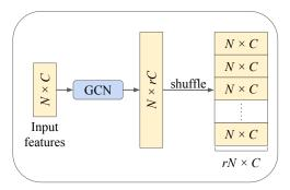
Figure 2: **Upsampling module: NodeShuffle.** We expand the number of input features by r times using a GCN layer, and then apply a shuffle operation to rearrange the feature map. r denotes the upsampling ratio.
