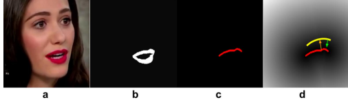
Figure 3. For a given image [a], we obtain the segmentation masks [b], its boundary [c] and distance transform (DT) image [d] of [c]. We employ a segmentation loss which tries to move the vertices on the projected mesh contour (yellow) to a lower energy position in DT. In addition, each pixel in the boundary (red) attracts the nearest vertex on the mesh contour.
