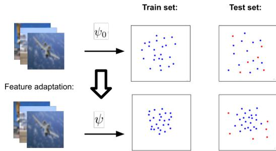
Figure 2: An illustration of our feature adaptation procedure, the pre-trained feature extractor  $\psi_0$  is adapted to make the normal features (blue) more compact resulting in feature extractor  $\psi$ . After adaptation, anomalous test features (red) lie in a less dense region of the feature space.
