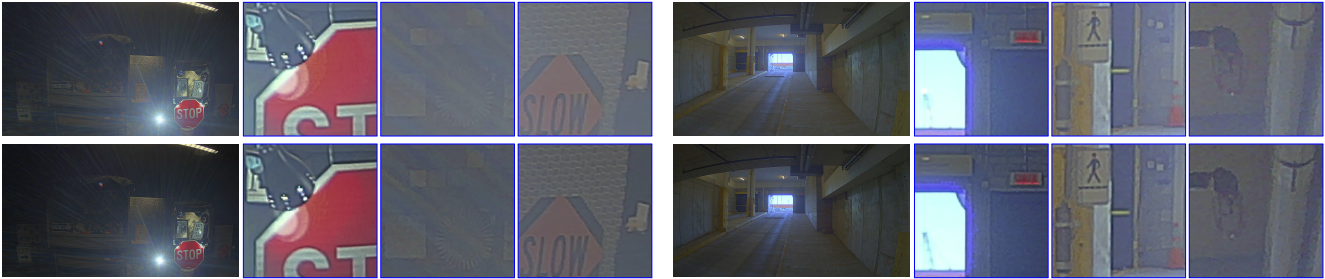
Figure 5: Results of ISP optimization for perceptual IQ. Left: HDR lab scene. Right: Real-life HDR scene. Top: Expert-tuned outputs. Bottom: Outputs of the proposed method. The proposed approach provides more detail and better dynamic range compression and local contrast. Please zoom into the electronic version of this document. Gamma correction applied to facilitate crop visualization.
