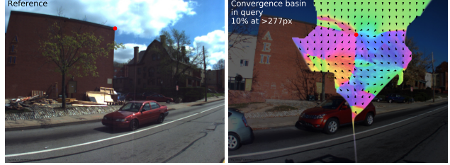
Figure 5. Wide convergence. For a red point in the reference image (left), we highlight in the query (right) the multilevel basin of attraction colored by the 2D gradient angle \partial \mathbf{F}_q / \partial \mathbf{p}_q^i \top \mathbf{r}_k^i . Deep features ensure a wide convergence despite appearance changes.
