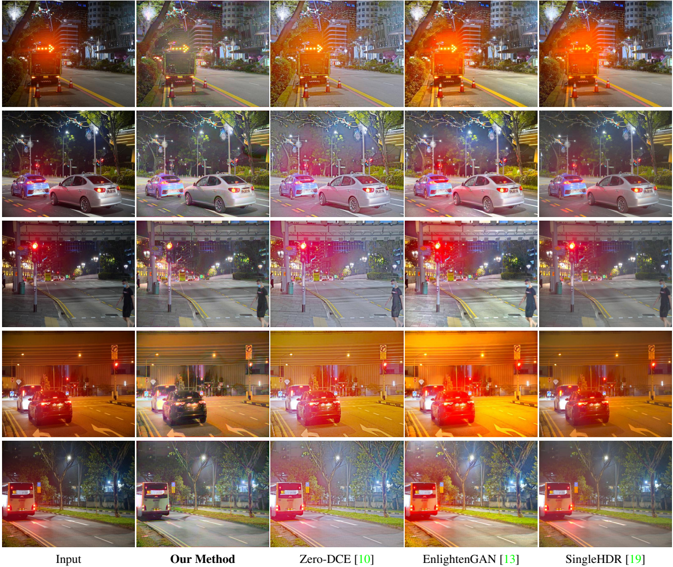
Figure 7. Qualitative results on the nighttime images with glow/glare/floodlight light effects. We can observe the better performance of our method compared to the baseline methods. Our result not only have the light effects suppressed but also increased dynamic range (e.g., better visibility in the low-light regions) which shows the effectiveness of our method for nighttime visibility enhancement.
