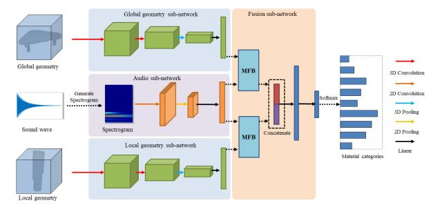
Figure 8. The network architecture of our proposed GLAVNet which consists of a global geometry subnetwork, a local geometry subnetwork, an audio subnetwork and a fusion subnetwork. After trained on our GLAudio dataset, GLAVNet can predict the fine-grained material categories based on the global geometry, the local geometry around the hitpoint and the sound.
