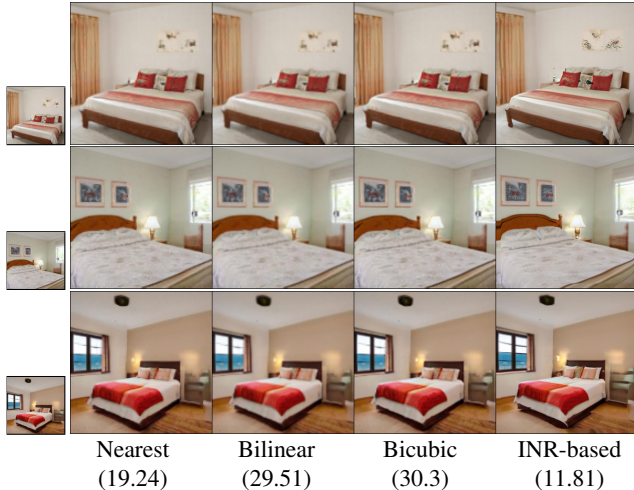
Figure 3: Out-of-the-box superresolution properties of the INR-based decoder. We train our INR-GAN on LSUN 128 \times 128 and perform upsampling at test time to 256 \times 256 resolution with either classical interpolation techniques (first 3 columns) or with “natural” INR-based upsampling by evaluating F_\theta on a denser coordinates grid. INR-based superresolution is much crisper and obtained without any additional supervision. Numbers in parentheses denote the corresponding UpsampledFID scores.
