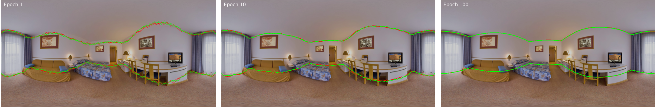
Figure 3. The evolution of HorizonNet as both the student (red lines) and teacher (green lines) over the course of training on 100 labeled and 1,009 unlabeled images. We encourage the student to learn layout representations of floor, ceiling, and wall boundaries from unlabeled data by enforcing consistency (or minimizing discrepancy) between student and teacher predictions perturbed by random model and data noise.
