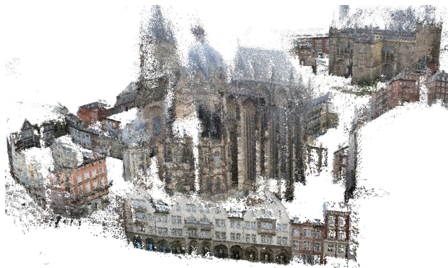
Figure 2. 3D reconstruction of Aachen [38] using the dense correspondences and uncertainties predicted by PDC-Net.
