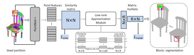
Figure 4: Network architecture of the PriorNet. After volumetric partitioning, each block is fed into the backbone network (PointNet++ [16]) to extract point-wise features. Two loss functions, similarity loss and low-rank loss, are devised to predict the segmentation result for the block.
