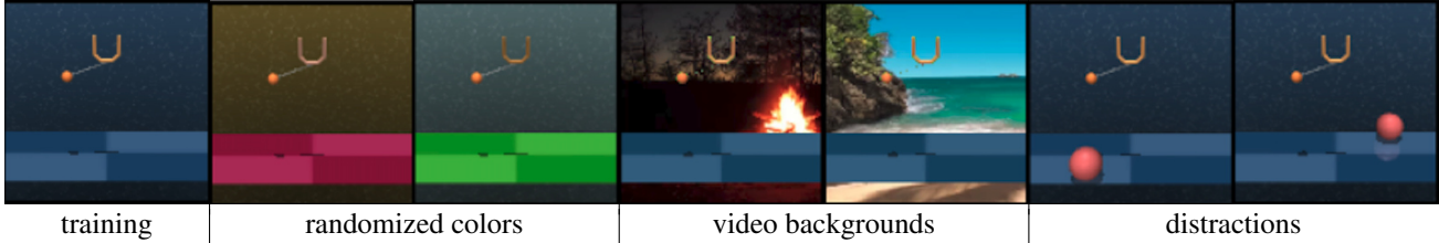
Figure 8: Visualization results of testing environments in DeepMind Control benchmark [15, 51]. The testing environment changes include randomized colors, video backgrounds, and background distractions.
