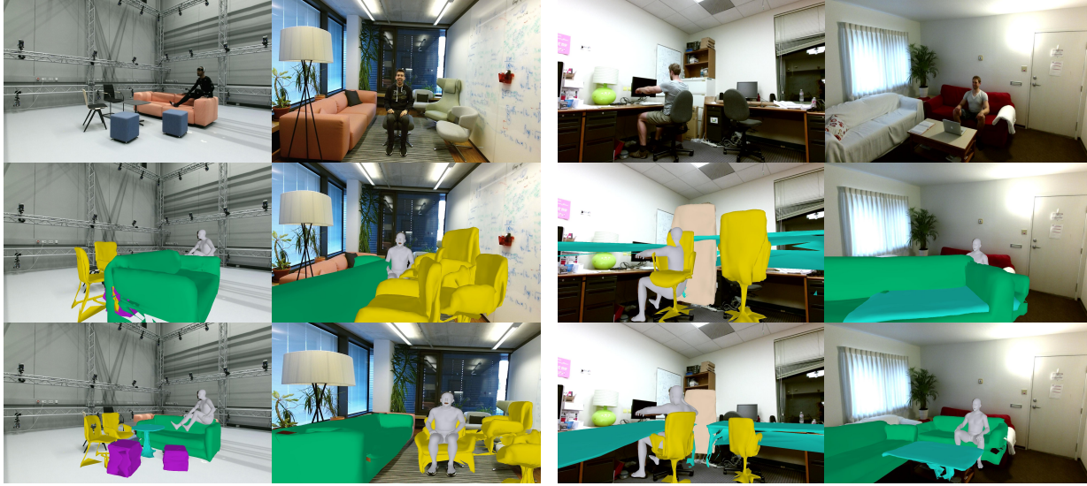
Figure 3. Left half: Qualitative results on PROX Quantitative and Qualitative datasets. The left frame is from PROX Quantitative. The right frame is from PROX Qualitative. Right half: Qualitative results on PiGraphs dataset. From top to bottom are the RGB input, the direct output from the scene and body mesh without any optimization, and the final mesh with the joint optimization.
