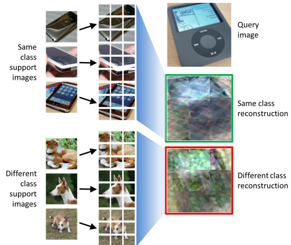
Figure 1. Visual intuition for FRN: we reconstruct each query image as a weighted sum of components from the support images. Reconstructions from the same class are better than reconstructions from different classes, enabling classification. FRN performs the reconstruction in latent space, as opposed to image space, here.
