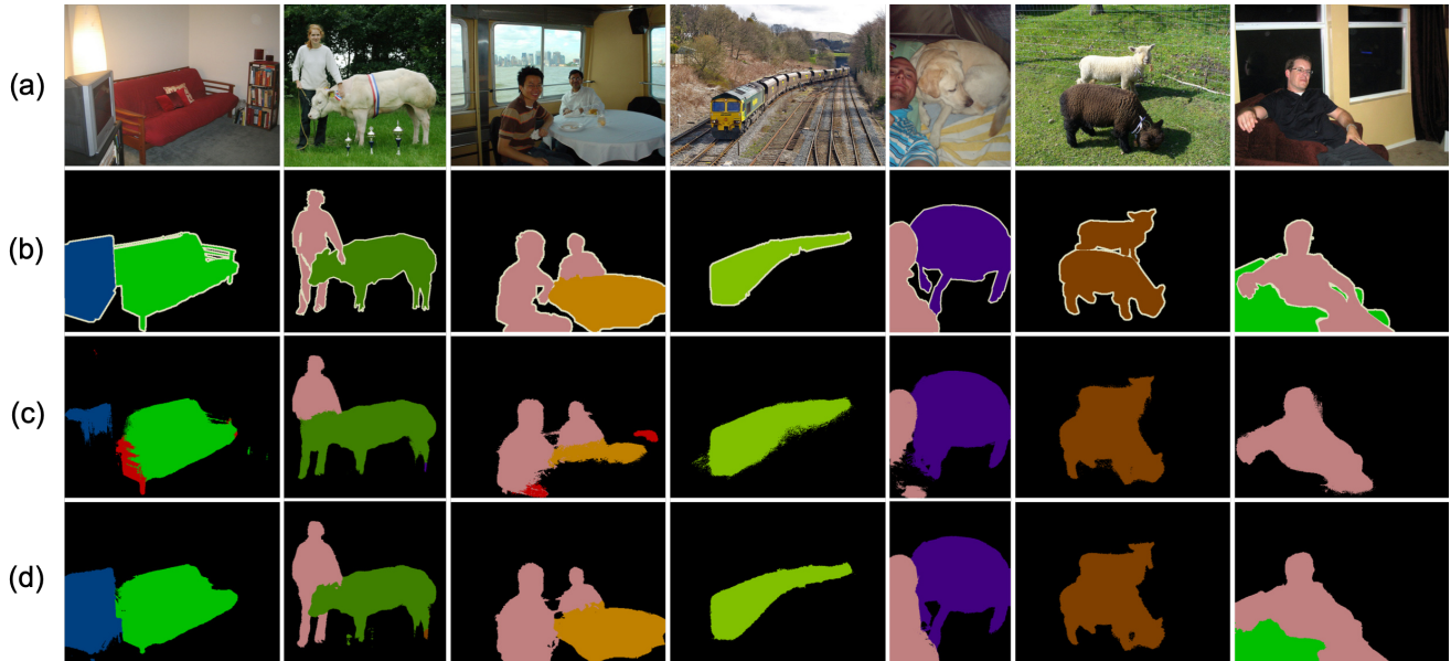
Figure 3. Qualitative segmentation results on PASCAL VOC 2012 validation set. (a) Original images. (b) Ground truth. (c) Segmentation results by [40]. (d) Segmentation results by DeepLab-LargeFOV model retrained on our pseudo-labels.
