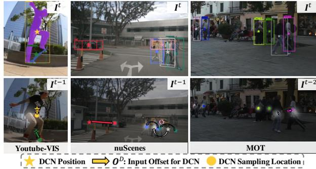
Figure 5. Visualization of DCN input offset  $O^D$ . The DCN kernel at  $\star$  is translated by  $\rightarrow$  and samples the previous feature at  $\bullet$ . For clear visualization, we only show the sampling center of the DCN kernel as depicted by  $\bullet$  in  $I^{t-\tau}$ . The previous image is highlighted by the previous class agnostic heatmap  $P_{agn}^{t-\tau}$ .
