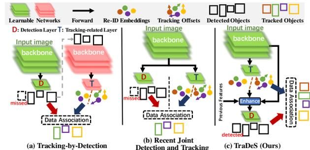
Figure 1. **Comparison of different online MOT pipelines.** Our method follows the joint detection and tracking (JDT) paradigm. Different from most JDT methods, the proposed TraDeS tracker deeply couples tracking and detection within an end-to-end and unified framework, where the motion clue from tracking is exploited to enhance detection or segmentation (omitted in the figure).
