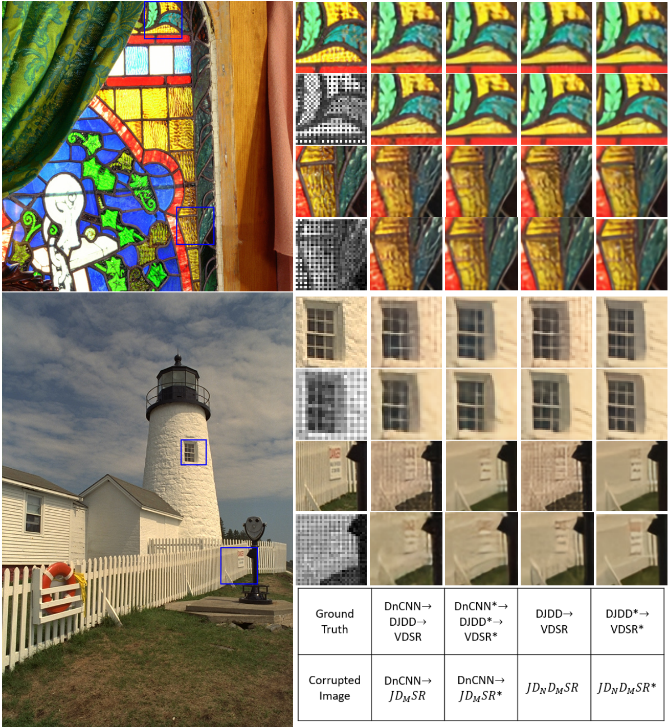
Figure 3: Visual comparison of the joint solutions of denoising, demosaicing and super-resolution. The scale factor is 2 and noise level is 10. The upper half part is the Image01 from McMaster dataset. The lower half part is the kodim19 from Kodak dataset. The sequence of ground truth image, corrupted image and resulting images corresponds to the illustration in the lower right corner.
