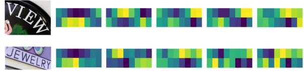
Figure 7. Feature maps before global average pooling of the pooling aggregator that learns n = 5 primitive representations. Values are averaged in the channel dimension for visualization.
