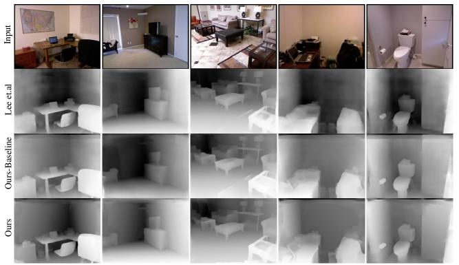
Figure 4. Qualitative comparisons between StruMonoNet and state-of-the-art monocular depth prediction approach(Lee et al.[23]) on NYUv2. Our approach exhibits salient gains over planar regions, including floor, wall, and the planar surface of furniture.
