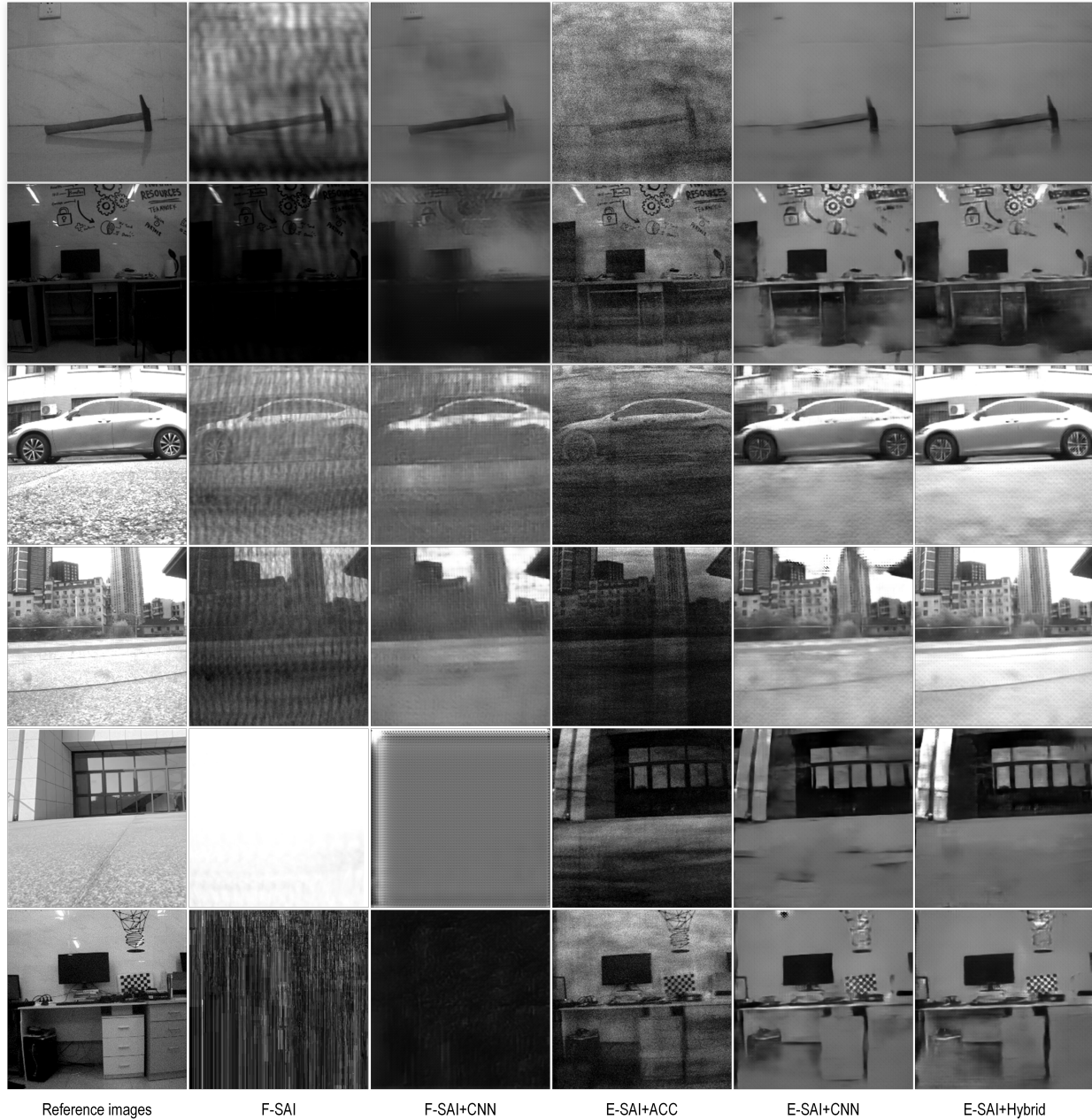
Figure 6: Qualitative comparisons between F-SAI and E-SAI algorithms under very dense occlusions (row 1-4) and extreme lighting conditions (row 5-6) for indoor (row 1,2 and 6) and outdoor (row 3-5) dataset.
