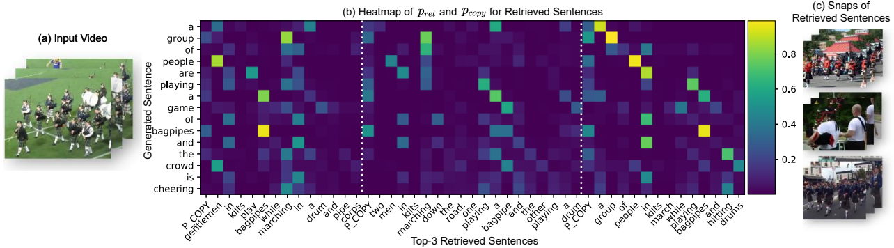
Figure 3. Illustration of the words copied from the retrieved sentences and their probabilities during the generation process. Each block represents the attention weights of the words in one retrieval sentence, and the first column of each block denotes the probability of copying.
