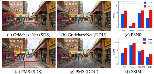
Figure 5. Qualitative and quantitative comparisons of 4K image processing strategies (SDS and DDU). The SDS scheme cannot consider global information and tends to generate artifacts.
