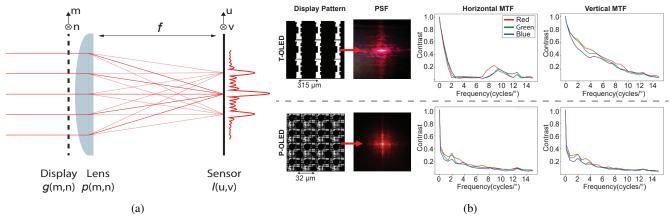
Figure 2: Image formation pipeline of under-display camera (UDC) problem. (a) Image Formation Pipeline. (b)Optics characteristics of UDC. The structure of the 4K T-OLED has a grating-like pixel layout. P-OLED differs from T-OLED in sub-pixel design. From left to right: Micrography of display patterns, PSFs (red light only) and MTFs (red, green, and blue).
