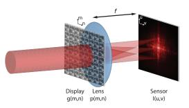
Figure 1: The newly proposed imaging system named Under-Display Camera (UDC). We mount display screen on top of a traditional digital camera lens. The design brings new trend of full-screen devices.
